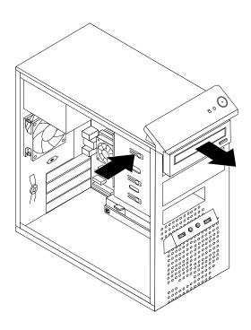
Figure 17. Removing the optical drive
